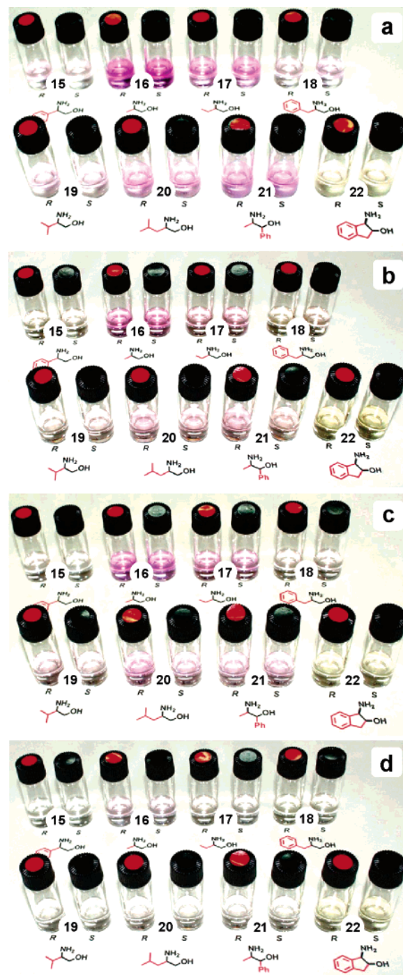
FIGURE 6. Color development by the hosts 2 – 5 with various \beta -amino alcohols. [hosts] = 5.0 \times 10^{-3} M, (a) host 2 , (b) host 3 , (c) host 4 , (d) host 5 . [guests 15 – 22 ] = 1.0 \times 10^{-1} M in \text{MeOH}/\text{CHCl}_3 = 9/1 at 0 °C. Red label on the lid denotes (R)-configuration of guest. Key: 15 , 2-amino-2-phenylethanol; 16 , 2-amino-1-propanol; 17 , 2-amino-1-butanol; 18 , 2-amino-2-phenylethanol; 19 , 2-amino-3-methyl-1-butanol; 20 , 2-amino-4-methyl-1-pentanol; 21 , erythro - \alpha -(1-aminoethyl)benzyl alcohol; 22 , cis -1-amino-2-indanol.
